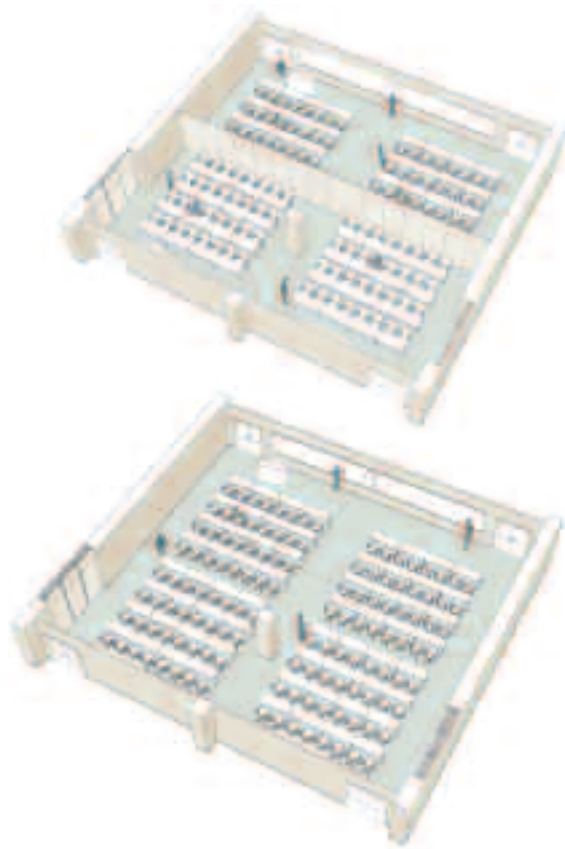
From one to four in a flash. Many classrooms in the new building can be transformed from one large room to two medium- or four small-sized classrooms in a matter of minutes.
