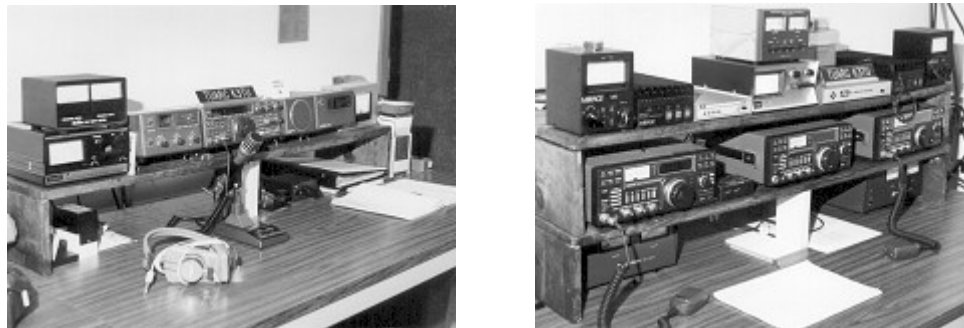
Figure 1. HF (left) and VHF/UHF/SHF (right) communication station equipment at TUARC K3TU.
