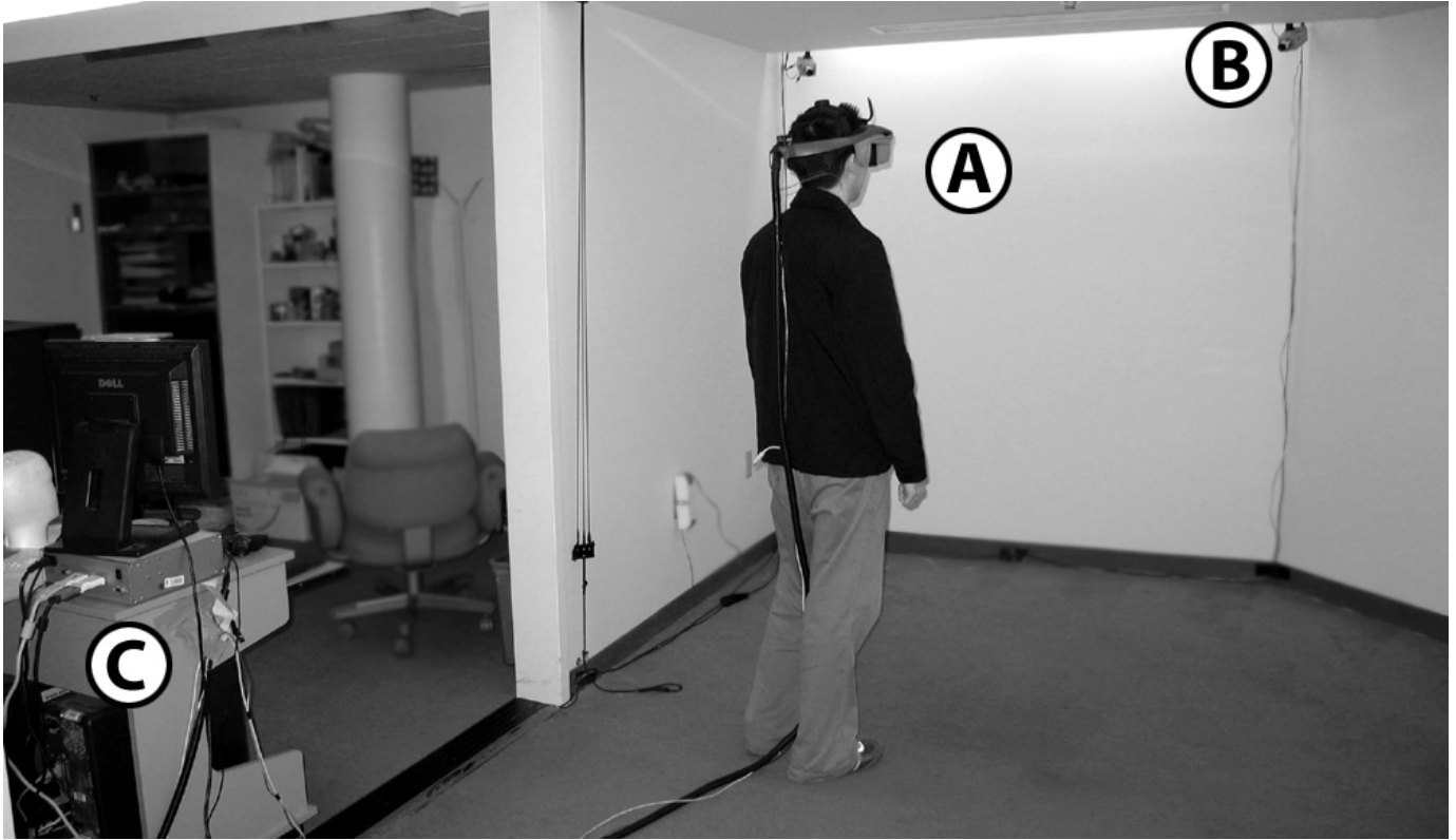
Figure 18 - Equipment setup: A) head-mounted display, B) tracking camera, C) rendering machine.
