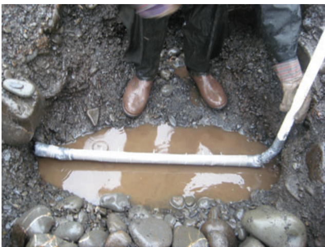
Figure 3. Photo of the Right (clean) Trench with the manifold placed across before refilling the trench. Note that the sediments were gravel and pebbles. The cobbles were mostly from the beach surface.
