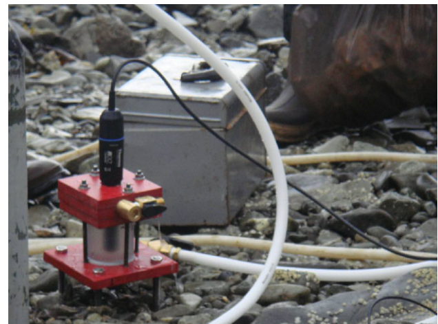
Fig. 5 Dissolved oxygen measuring setup during operation. The DO probe (black) is immersed in the measuring chamber (transparent cylinder with red top and bottom)
