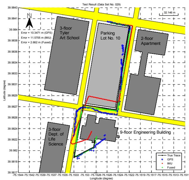
Figure 6. Comparison of GPS, IMU and Fused Data.
