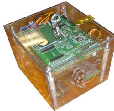
Figure 5. Prototype for Micro-Navigation Sensor.
