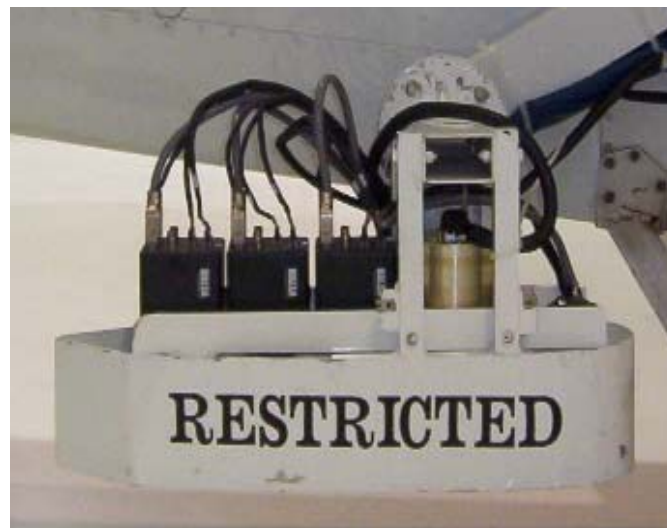
Figure 6. Three airborne cameras (black boxes on the left) and an inertial measurement unit (light colored cylinder on the right).
