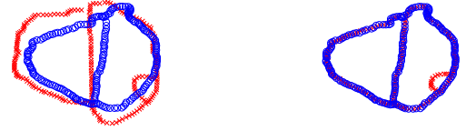
Fig. 5. The landmarks point sets before registration (left) and after registration using ROI estimation method (right) in CT image / Laser Scanner image experiment.
