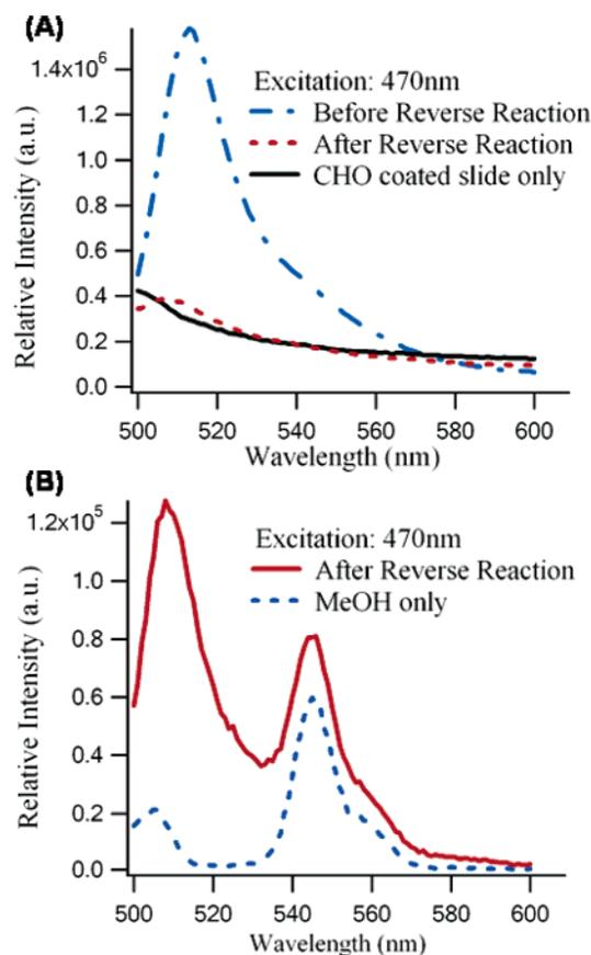
**Figure 5.** (A) Fluorescence detections of D2371- reacted slide AL (aldehyde-coated) before and after reverse reaction. (B) Fluorescence detection of the solution after reverse reaction.
