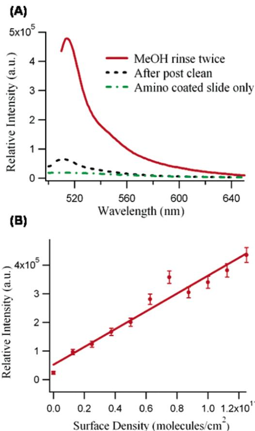
**Figure 3.** (A) Fluorescence detection of two D2183-reacted amine-coated slides. One sample is only rinsed in MeOH twice after the reaction (red solid line), the other sample is subjected to the full postreaction cleaning procedure (black dash line). The dashed-dotted line is the intrinsic fluorescence of the clean amine-coated slides. (B) Calibration curve for dye D2183 (Scheme 1). All samples were excited at 470 nm.
