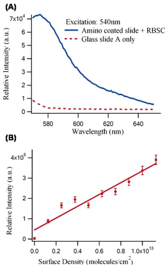
**Figure 2.** (A) Fluorescence detection of RBSC-reacted glass slide A (amine-coated) and intrinsic fluorescence of glass slide A (dashed line). (B) Calibration curve for fluorescence at 580 nm from RBSC on glass slide A.
