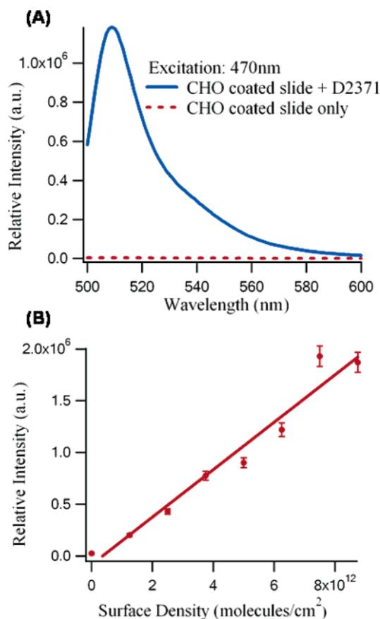
**Figure 4.** (A) Fluorescence detection of D2371- reacted glass slide AL (aldehyde-coated) and unreacted AL glass slide (dashed line). (B) Calibration curve for dye D2371 (Scheme 1), excited at 470 nm.
