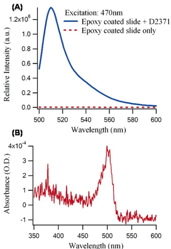
**Figure 6.** Fluorescence detection (A) and UV–vis detection (B) of D2371-reacted glass slide E (epoxy-coated).
