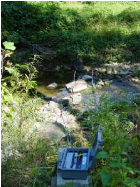
Data logger at Terwood Run, measures water level, conductivity and temperature
